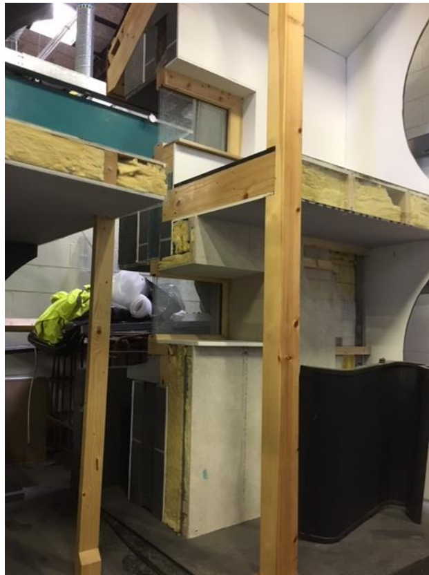
Figure 29: Model constructed depicting cavity block wall with (a) internal insulation and full-fill cavity on the lower level and (b) external insulation with full-fill cavity on the higher level.
