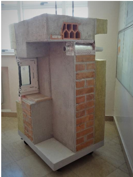
Figure 10: Model of the external insulation on the existing masonry wall
