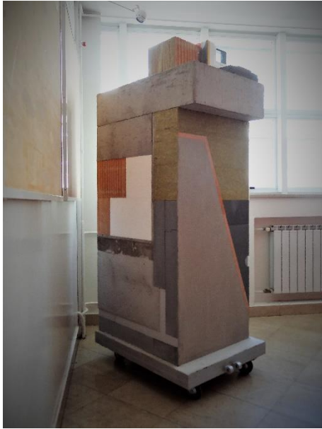
Figure 11: Model of the foundation detail (external insulation) and balcony detail (thermal break)
