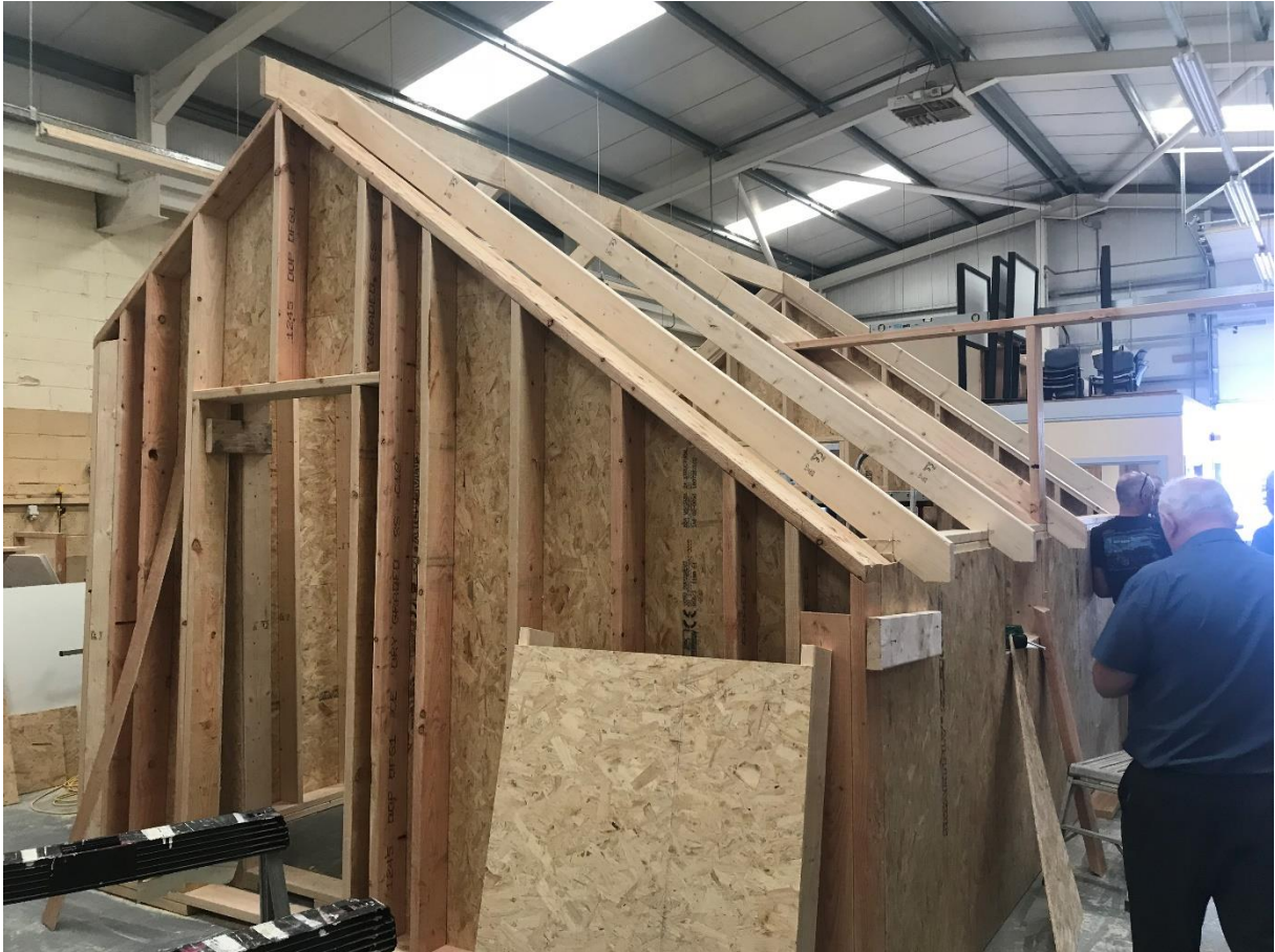
Figure 32: Airtight room for airtightness testing
