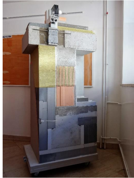
Figure 11: Model of the foundation detail (external insulation) and balcony detail (thermal break)
